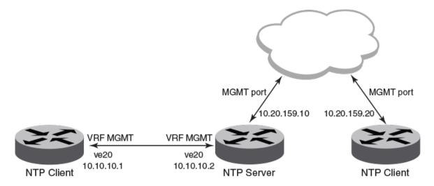
In this scenario, the NTP server has one client using Management VRF and one client on a management port.
