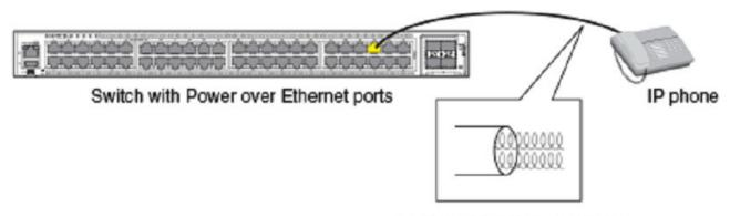
Power and data signals travel along the same pairs of wires at different frequencies.
